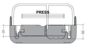
Depending on the used flaps of the terminal following cable jacket diameter difference between the side D2 and D1 terminals is recommended:
