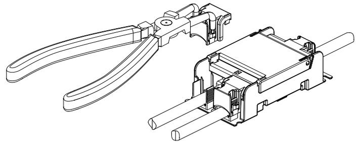
1. Insert release tool device into cut-out, e.g. KNIPEX 46 21 A21 Seeger ring pliers or screwdriver
