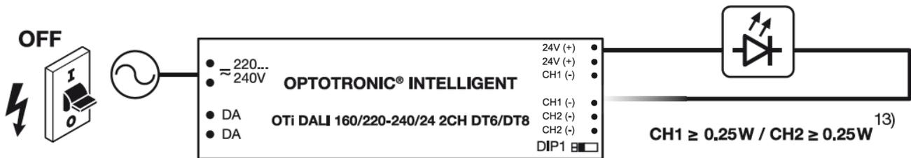
1. Connect the LED loads to the desired channels from 1 to 2.
