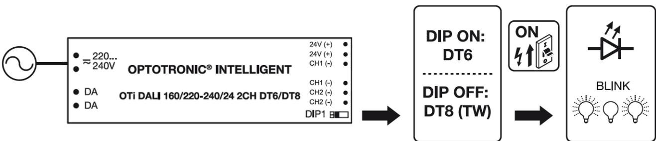
3. Connect the ECG to the mains: the LED loads start blinking.
