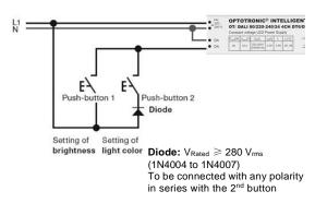
This driver supports single and double button Touch DIM operation. The 2<sup>nd</sup> button must be connected in parallel with the 1<sup>st</sup> by means of a diode.
