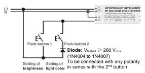
This driver supports single and double button Touch DIM operation. The 2<sup>nd</sup> button must be connected in parallel with the 1<sup>st</sup> by means of a diode.
