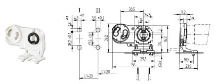
L1-20: Recommended dimension - The distance between the cut-outs and the tolerance should be governed by the dimensions of the respective lamps and luminaires.
