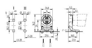
L1-20: Recommended dimension - The distance between the cut-outs and the tolerance should be governed by the dimensions of the respective lamps and luminaires.
