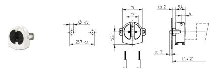
L1+20: Recommended dimension is based on use of one lampholder with and one lampholder without spring. The final distance should be governed by the dimensions of the respective lamps and luminaires.
