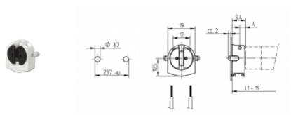
L1+19: Recommended dimension - The distance between the cut-outs and the tolerance should be governed by the dimensions of the respective lamps and luminaires.
