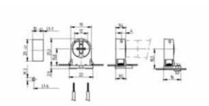
L1-1 / L1-6: Recommended dimension - The distance between the cut-outs and the tolerance should be governed by the dimensions of the respective lamps and luminaires.
