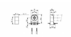
L1-1: Recommended dimension - The distance between the cut-outs and the tolerance should be governed by the dimensions of the respective lamps and luminaires.
