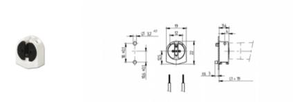
L1+19: Recommended dimension - The distance between the cut-outs and the tolerance should be governed by the dimensions of the respective lamps and luminaires.
