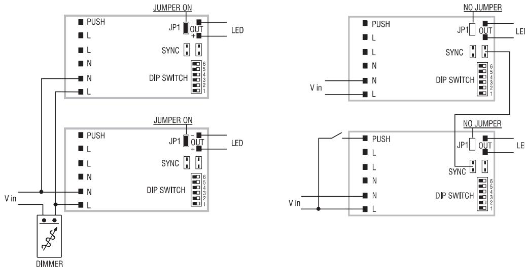
**PHASE-CUT dimming** - To avoid flickering, keep the slaves at 100% dimming level.
