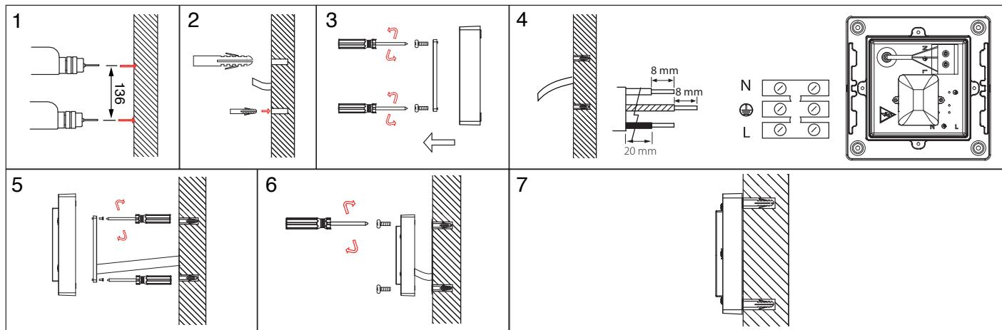
Uppoasennus | Infälld montage | Recessed mounting
