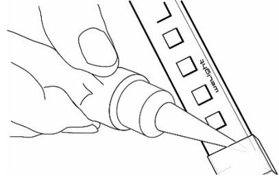
Use the included Silicon Tube to dispense silicon around the end of the LEDtape to facilitate the insertion into the connector sleeve.
