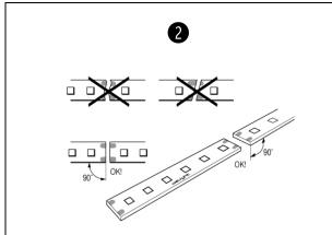
Always cut the LEDtape in a straight line  $-90^{\circ}$  in relation to the PCB edges. Failure to do so can result in damage of the internal conducting paths. Use Welight's official connection accessories to split, connect, bridge and re-seal the LEDtape.
