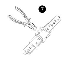
Use a pair of flat pliers to press down on each side of the cap until they lock in position. A "CLICK" can be heard when the pins are locked.
