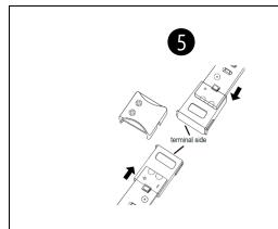
Push the lubricated ends of the LEDtape all the way into the sleeves.
