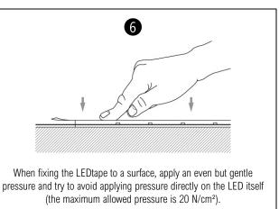
After assembly always check that the entire length has attached properly to the surface and that there is no air pockets underneath.
