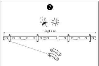
If the total length is longer than 2 meters or when used in environments with large variations in temperature (e.g. outdoor applications) it is recommended to use the included screw mounting clips in addition to the adhesive tape.
