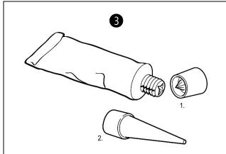
Locate the accessories included in the LEDtape box. Puncture the seal of the tube using the backside of the tube cap. Screw the dispersion needle onto the tube. Cut the top of the needle at an angle of 45-60°.
