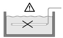
Do not use connectors permanently under water! When using connectors, the overall protection of the LEDtape will be reduced from IP68 to IP67.
