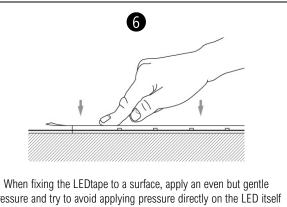
pressure and try to avoid applying pressure directly on the LED itself (the maximum allowed pressure is 20 N/cm<sup>2</sup>).
