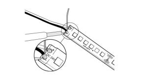
If you need to solder the LEDtape, pre-tin the cables only. Soldering temperature max 300 °C for 4 seconds.
