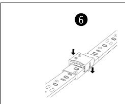
Put the bridge connector on top of the sleeves and push downwards.
