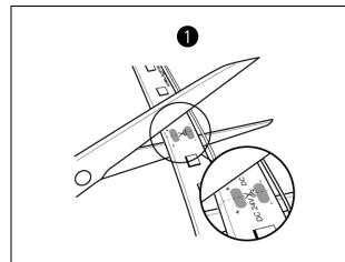
The LEDtape is separable at the middle of every solder pad with the full function of each LED segment. It is only allowed to cut at the indicated cutting line.
