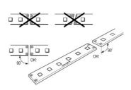
Always cut the LEDtape in a straight line  $-\,90^\circ$  in relation to the PCB edges. Use Welight's official connection accessories to split, connect, and bridge the LEDtape.
