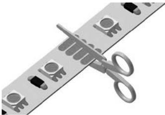
Cut the LEDtape in the middle of the solder pads.
