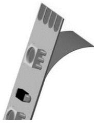
Peel off approx. 1 cm of the adhesive tape from the back of the LEDtape.
