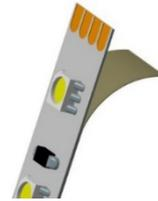
Peel off approx. 1 cm of the adhesive tape from the back of the PCB.
