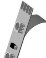
Peel off approx. 1 cm of the adhesive tape from the back of the LEDtape.
