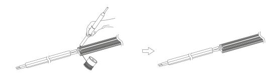
5. Put the plug on the line and repeat the gluing steps as shown in Figure 2. Then plug the lamp strip into the plug and complete the installation, as figure 5.
