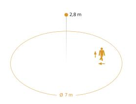
Possible mounting height: 2,00 m – 4,00 m Orange: radial and tangential **Dimension Drawing**
