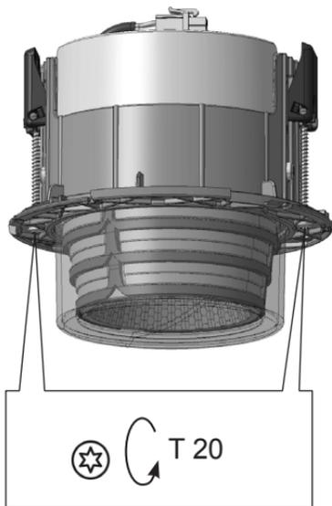
remove screws and lever parts
