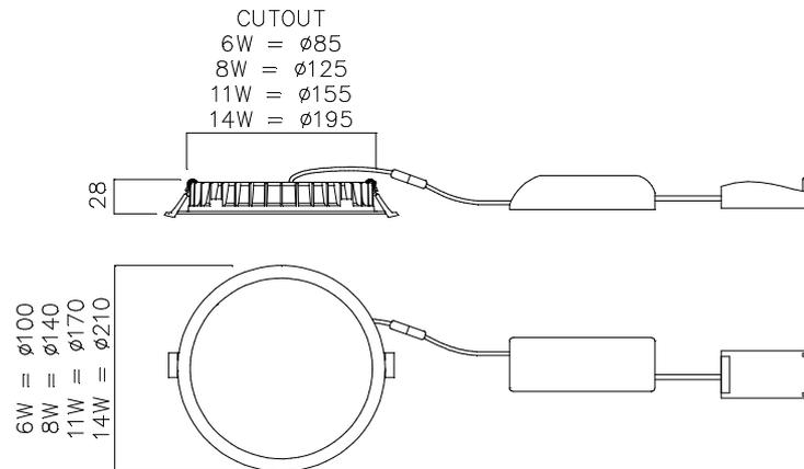
1. Decide the mounting position in ceiling & cut a round hole to the required diameter (see diagram). Care should be taken when cutting the hole to avoid structures & to not exceed the specified cutting diameter so as not to expose the cut edge.
