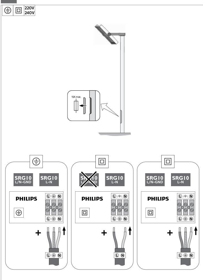
(EN) 10kV extra surge protection (SRG10) is ensuring Differential mode protection.
