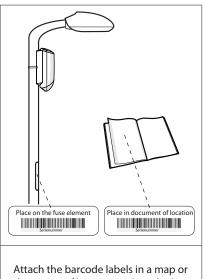
Attach the barcode labels in a map of document of location and inside the service hatch or on pole.
