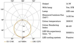
14 W Yes, STEINEL LED system LED cannot be replaced 1430 lm 3000 K 80-89
