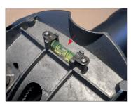
8. Check bubble tube and adjust the luminaire.
