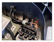
5. Connect cable to the terminal. 2x1mm²—▶2x2,5mm².
