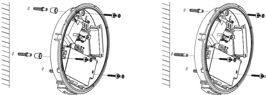
4: **a.** Connect the plugs between the battery and driver if with emergency function. **b.** Choose the power with DIP switch if it's the wattage changeable version (12 inch only). **c.** Connect the AC wires to the block.
