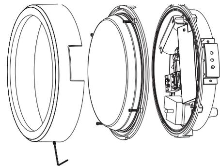
3: Fix the back housing on the wall or ceiling by screws.
