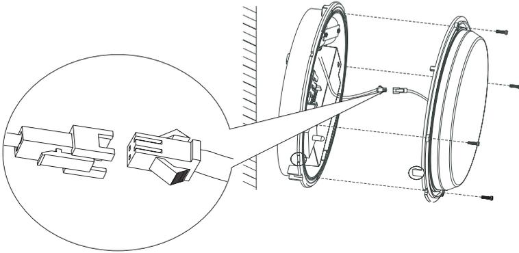
6: Buckle the frame back and fix it by proper tools.
