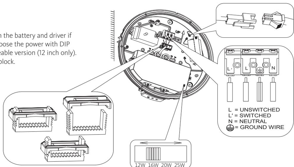
5: Connect the DC plugs, put back the cover to the back plate and fix it by the screws.
