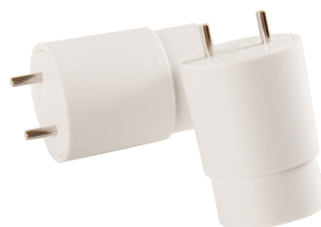
Lampholder adapter T8 to T5 for Aura UltiLED Protector Long Life. Note that the lampholder adapter only fits 1149 and 1449 mm tubes.
