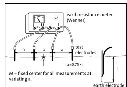
Measurement of earthing resistivity.
