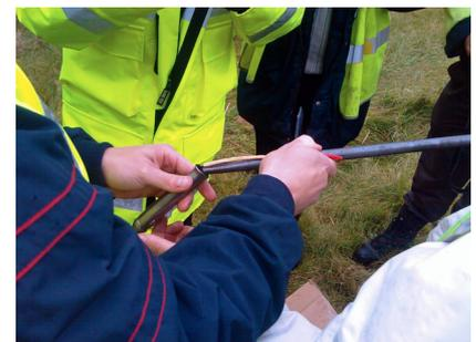
*The earthing wire locks in the hardened steel tip with the leading rod.*
