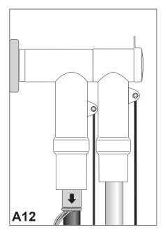
Ensure that the grounding lead of the housing is fastened tightly.
