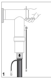
Remove from the installed connector the conductive endcap and save it in a clean container.
