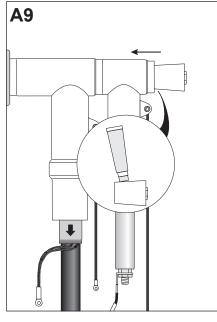
a. Place a string into the rear entry of the connector as shown.
