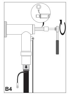
Insert coupling stud with tinned Cuwasher (see detail) into the rear end of the connector and tighten it up with a torque wrench (27 mm).
