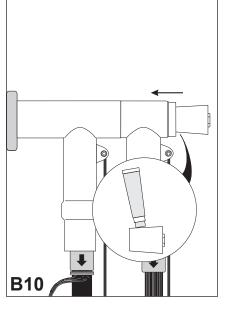
Clean the inner surface of connector back end and apply a thin layer of assembly lubricant. Do the same with the conical interface of the back plug as shown in detail.
