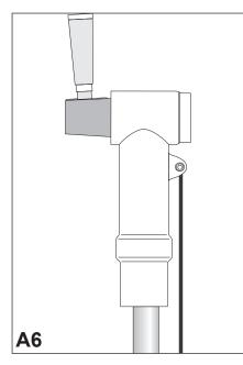
Clean the conical front end of the surge arrester and apply a thin layer of lubricant onto the outer surface of the cone with the sponge top. Continue **immediately** with the next step.
