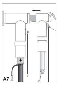
Align the conical front end of the surge arrester with the rear end of the already installed connector and push the coupling connector in position.
