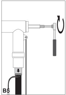
**Insert a new threaded pin M16 marked EXRM-1885** into the rear end of the coupling stud and tighten it up with an Allen key (8 mm). Maximum torque: **30 Nm**.
