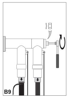
Insert the spring washer and hex nut. Tighten the hex nut onto the stud with a torque wrench (24 mm) at a torque of **30 Nm**.
