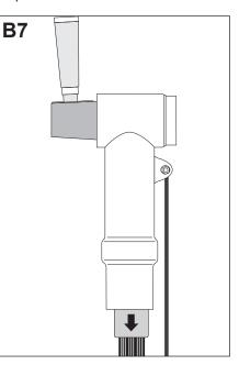
Align the conical front end of the coupling connector with the rear end of the already installed connector and push the coupling connector in position.
