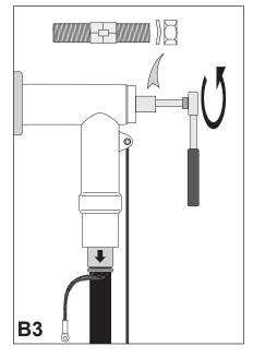
**Remove** from the installed connector **hexagon nut, washer, threaded pin** and save it in a clean container.
