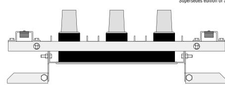
The ELASTIMOLD (K)1501J3-U-8 junctions are designed to provide a means of apparatus changeout, sectionalising, tapping or looping.
