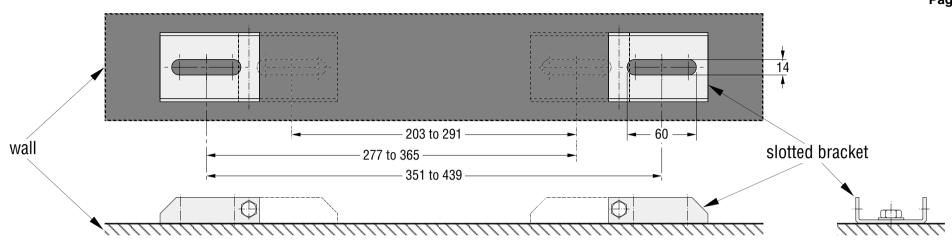
1. Remove slotted mounting brackets from assembly and attach to wall with suitable fasteners.
