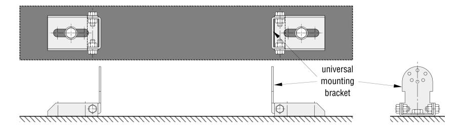
2. Install the universal mounting brackets on to the slotted brackets.
