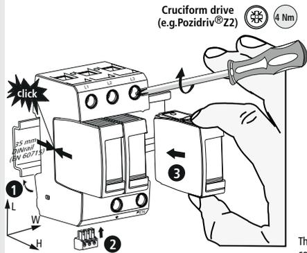
There is no distance from the SPD to any earthed conductive surface required. /
