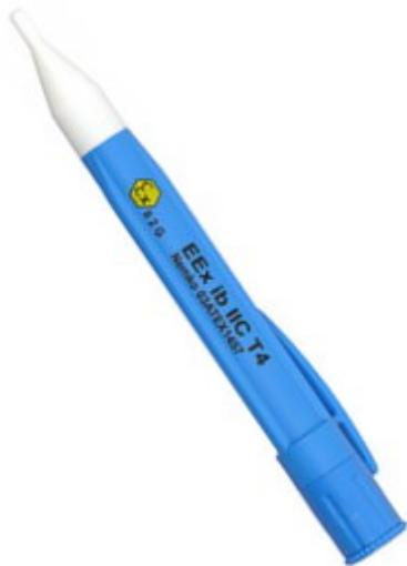
The EEx approved Magnet Stick is an instrument for testing for the presence of magnetic fields. By simply holding the tip of the instrument near the test area, it indicates a magnetic field by glowing. The test lamp responds to all kinds of magnetic fields, from alternating current to direct current and permanent magnets. (Sensitivity 300 gauss 0,3 mT). The ATEX and IECEx approvals are confirmed by NEMKO. (II 2G EEx ib IIC T4) **General Features:**
