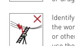
Identify all risks posed by electrical equipment in the working area, e.g. high-voltage power lines or other exposed electrical equipment. Do not use the ladder if there are electrical risks.
