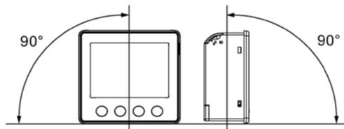
Figure 3-1 Mounting position
