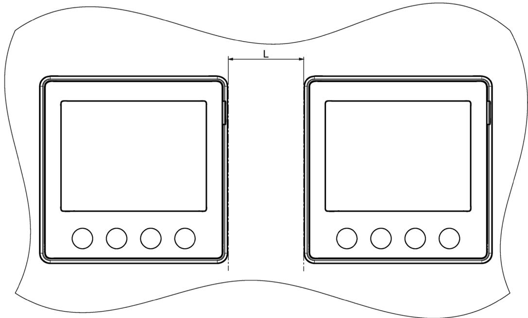
L = 5 mm if compact brackets available to order as separate components are used (article number: 7KM9900-0GA00-0AA0)
