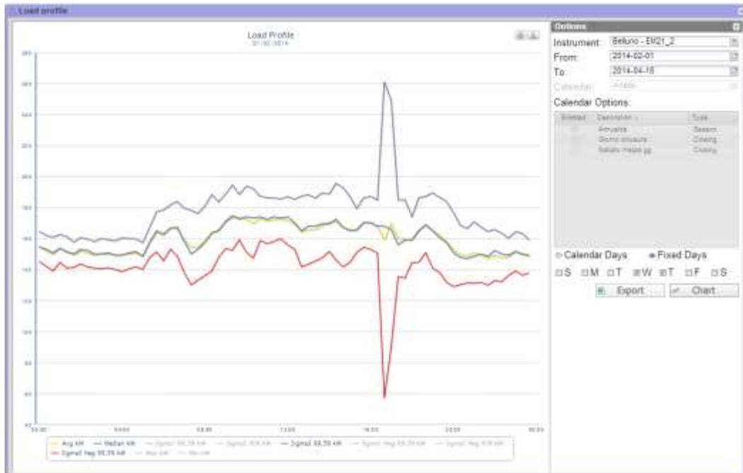
Figure 22: Load profile menu with days of analysis picked from the calendar
