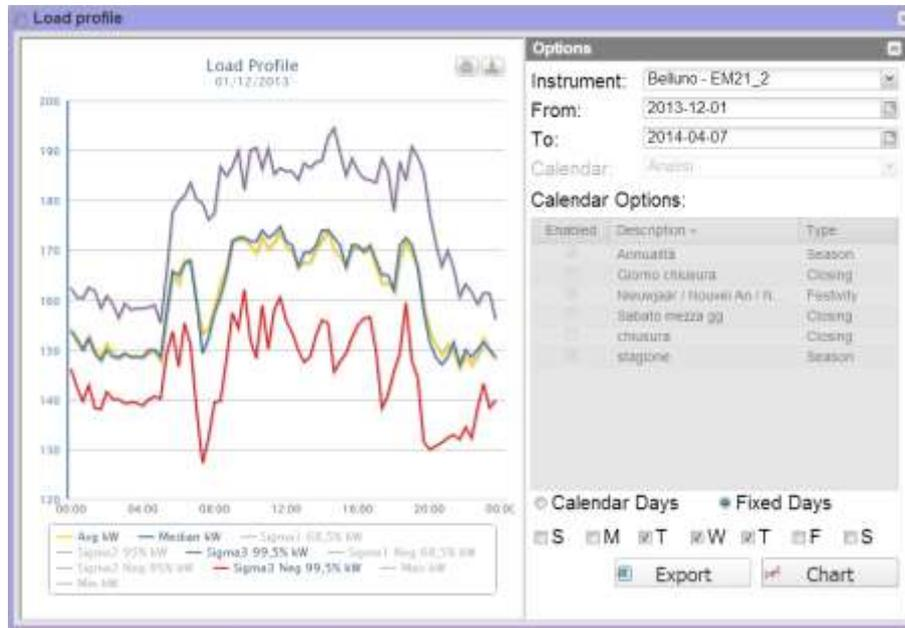
**Figure 23: Load profile menu with manually selected days**
