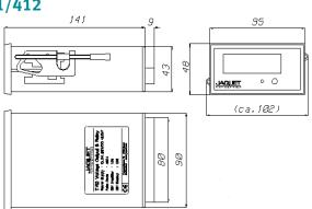
Rail DIN 4622713 (EN 50022) or mounting plate to DIN 43660 (46121)
