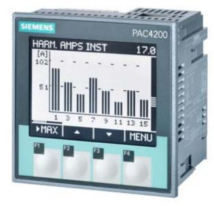
SENTRON, measuring device, 7KM PAC4200, LCD, L-L: 690 V, L-N: 400 V, 5 A, 3-phase, Modbus TCP, optional Modbus RTU / PROFINET / PROFIBUS / DI/DO, apparent/active/reactive energy / cos phi, harmonics: 3.-31., THD, class 0.2 acc. to IEC61557-12 or cl. 0.2S acc. to IEC62053-22, wide-range pwr sup. unit AC/DC, screw terminals
