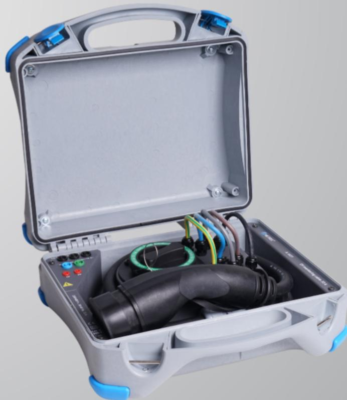
The A 1631 EV monitoring cable is a special accessory designed for CP signal, current and voltage monitoring during Electric Vehicle (EV) charging process in conjunction with supported Metrel testers and adapters. It is equipped with a Type 2 female plug connector to connect to an EV and a Type 2 male socket outlet for connecting to Electrical Vehicle Supply Equipment (EVSE).
