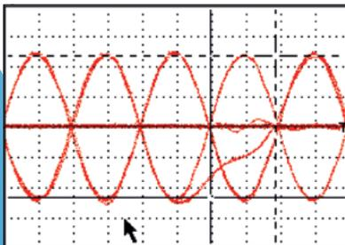
**Eye diagram:** an advantage for recurrent data display. The traces are cumulated on screen, alternating the trigger-edge polarity.
