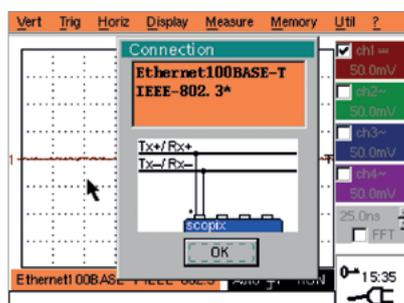
SCOPIX BUS proposes help with connection according to the bus to be checked, with the corresponding wiring diagram.
