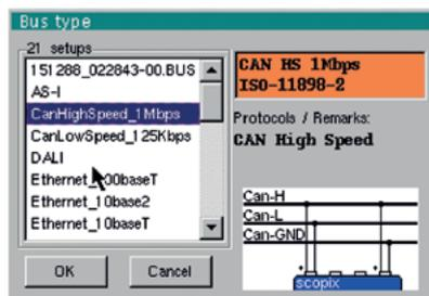
14 buses, 21 available configurations and several protocols (IP, TCP, Modbus, Profinet, etc.) selectable from a drop-down menu and already integrated in the SCOPIX BUS models.
