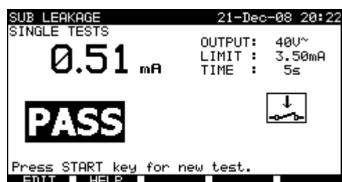
Example of substitute leakage current measurement results
