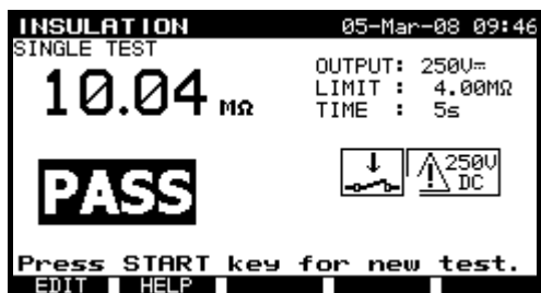
Examples of insulation resistance measurement results
