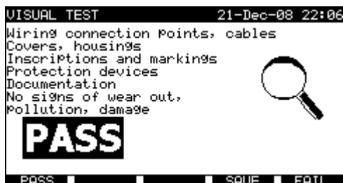
Examples of visual test measurement results
