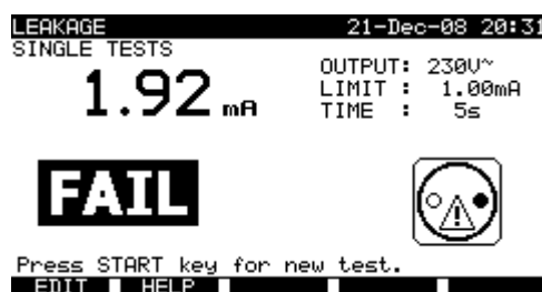
Examples of differential current measurement result
