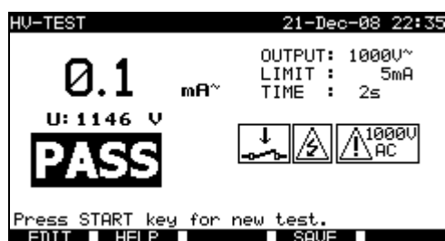
Examples of high voltage withstanding test results
