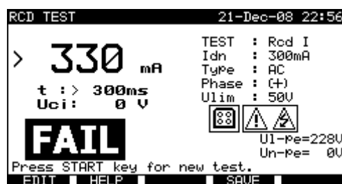
Examples of RCD trip out current measurement results
