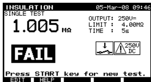
Examples of insulation resistance measurement results
