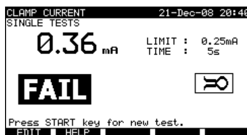
Examples of clamp current measurement result
