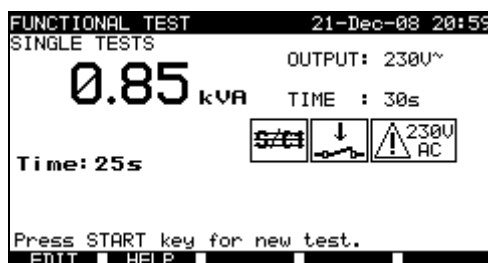
Example of apparent power measurement result
