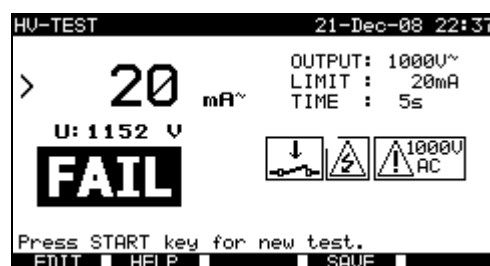
Examples of high voltage withstanding test results
