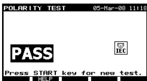
Examples of polarity test result
