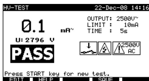
Examples of high voltage withstanding test results
