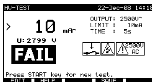
Examples of high voltage withstanding test results
