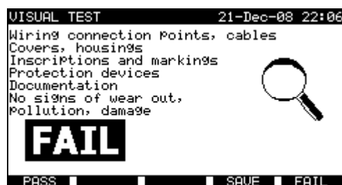
Examples of visual test measurement results
