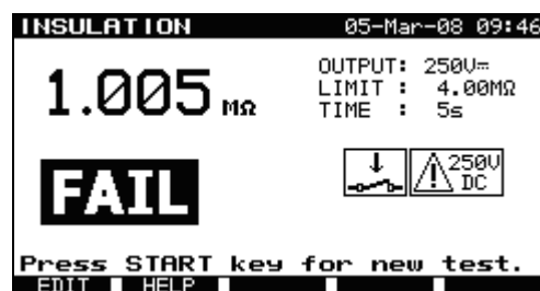
Examples of insulation resistance measurement results
