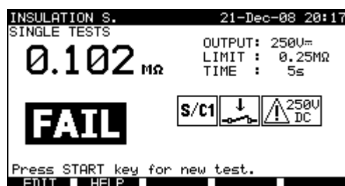
Example of insulation S. resistance measurement results
