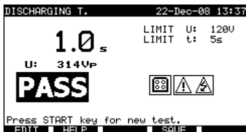
Examples of discharging time measurement results
