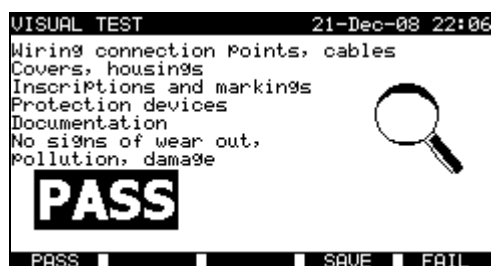
Examples of visual test measurement results
