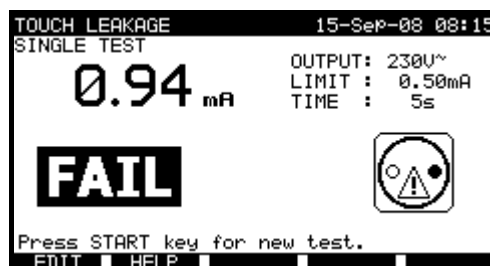
Examples of touch leakage current measurement results
