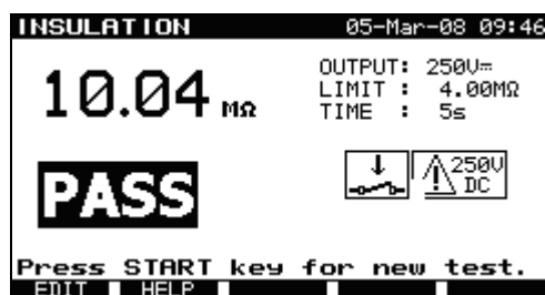
Examples of insulation resistance measurement results
