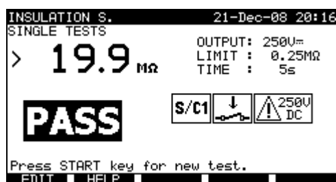
Example of insulation S. resistance measurement results
