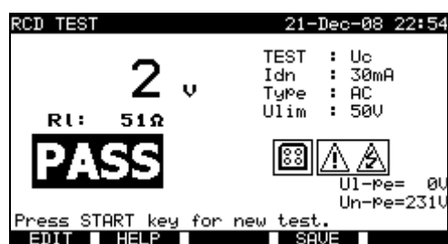
Example of contact voltage measurement results
