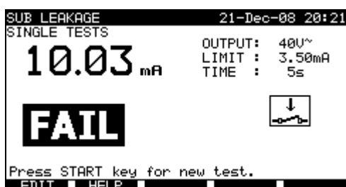
Example of substitute leakage current measurement results
