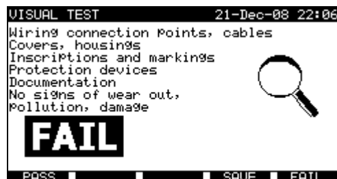
Examples of visual test measurement results
