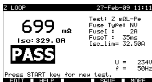
Example of Z mΩL-Pe loop measurement results
