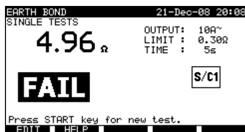
Examples of earth bond resistance measurement results
