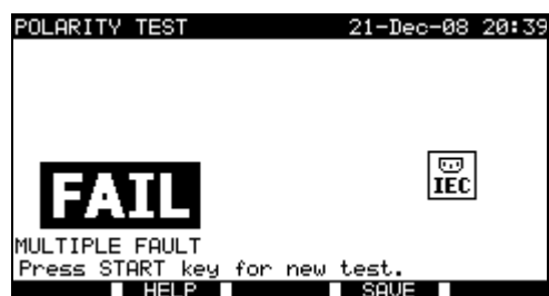
Examples of polarity test result
