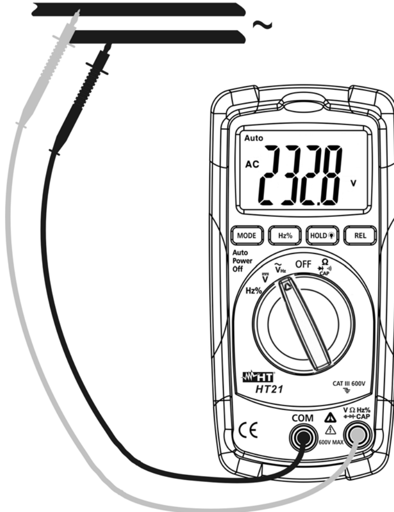
Fig. 3: Using the instrument for AC voltage measurement
