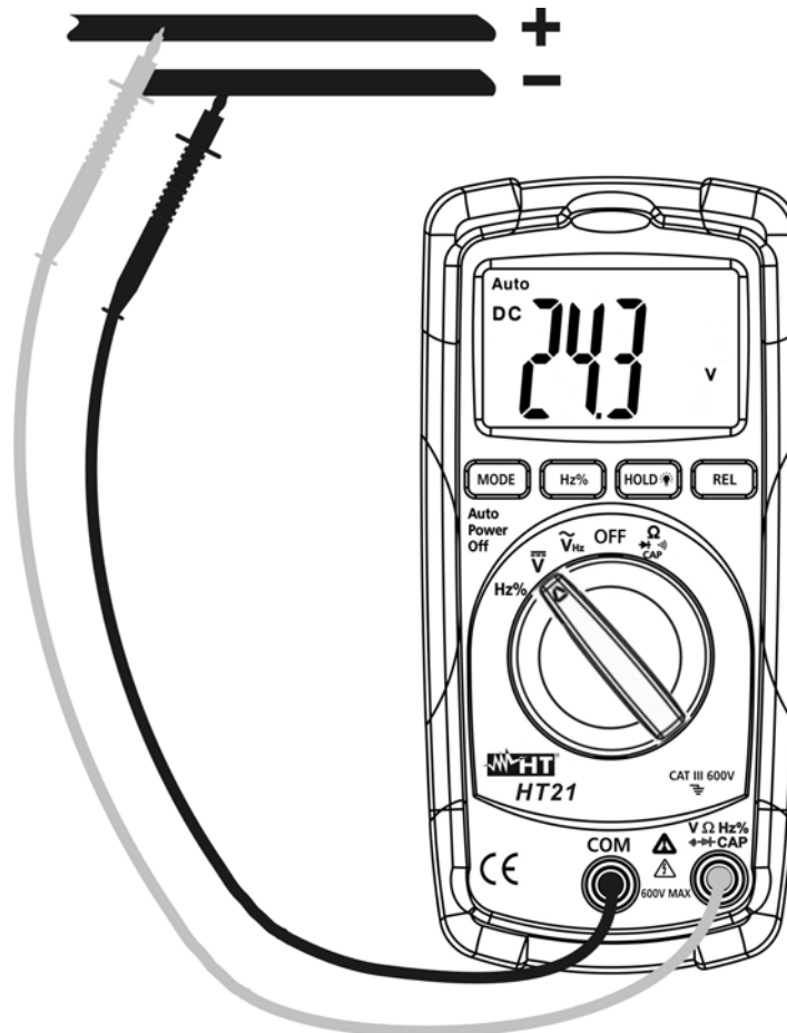
Fig. 2: Using the meter for DC voltage measurement
