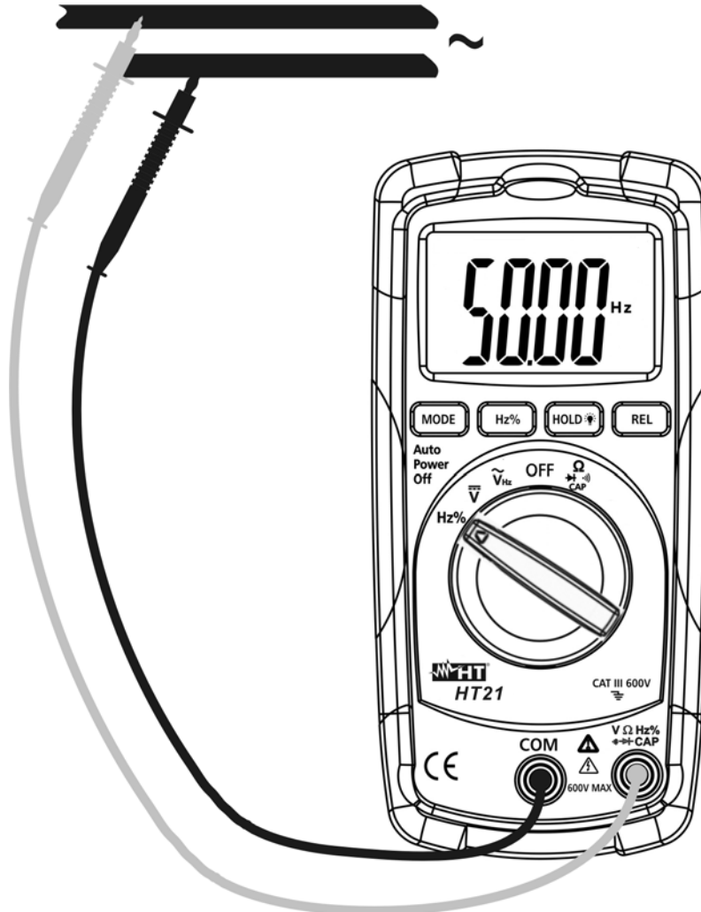
Fig. 6: Using the instrument for frequency and duty cycle measurements
