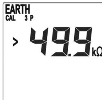
6. If the volt metric circuit (terminal S) shows a too high resistance value the side message is displayed.
