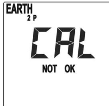
4. When measuring, if terminals' voltage is higher than **6V**, the instrument does not effect the test. A long sound tone is emitted indicating an anomalous condition and the side screen is displayed for 5 seconds (S-E indicates between which inputs voltage was detected), then the instrument displays the initial screen.
