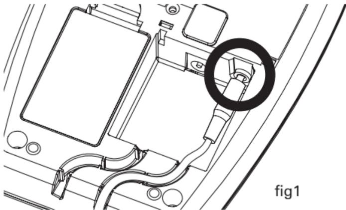
2. Remove the battery cover on the back of the Strobe by pulling back the clip to release. Connect the rechargeable battery, by aligning the terminals (red wire to red wire) and pushing the connectors together. You may hear the Strobe beep twice as you do this.
