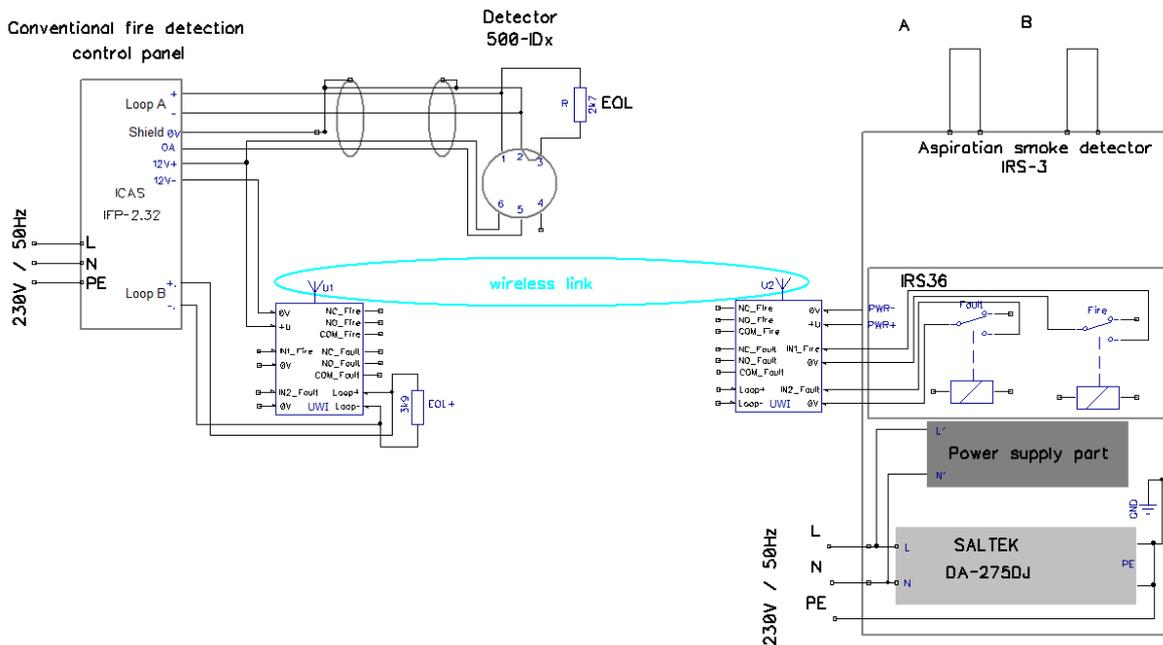
ICAS conventional pane IFP-2.32 and IRS-3 wireless connection by UWI with fire and fault indication in the loop B.
