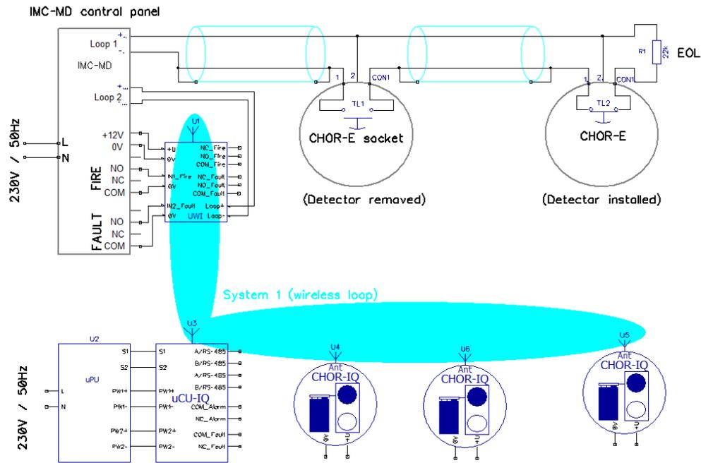
The IMC-MD system is wireless connected by UWI as one detector/node into uCU-IQ system (another CHOR-IQ alike)
