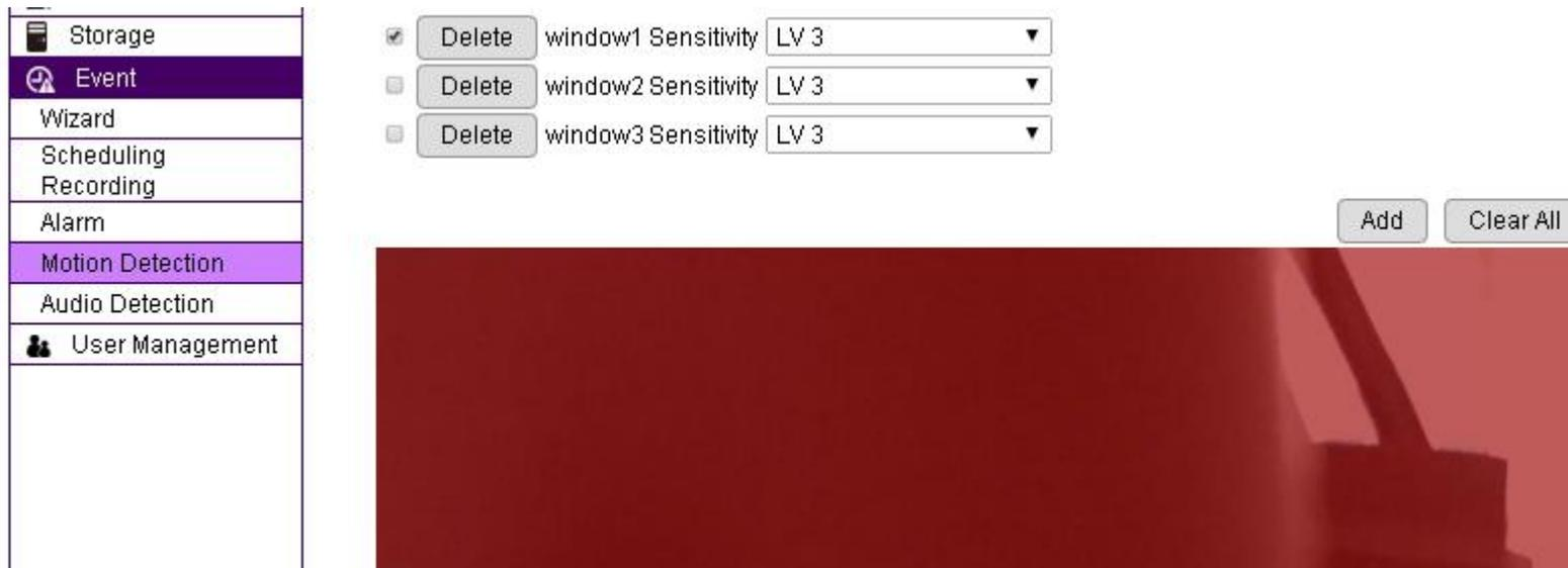
The screenshot displays a web-based configuration interface for a camera. On the left is a vertical navigation menu with the following items: Storage, Event (highlighted in purple), Wizard, Scheduling, Recording, Alarm, Motion Detection (highlighted in light purple), Audio Detection, and User Management. The main content area shows three motion detection windows, each with a 'Delete' button and a sensitivity dropdown menu set to 'LV 3':
