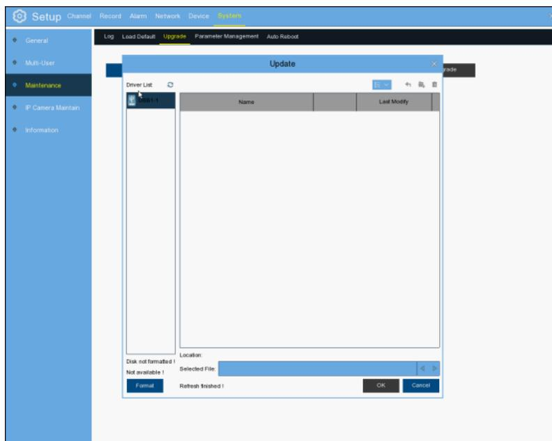
1. Copy the firmware file (.sw file) to your USB drive, and insert the USB flash drive into the NVR's USB port.
