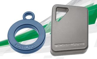
ROSSLARE'S PROXIMITY CREDENTIAL TAGS ARE HIGHLY COMPACT AND SLEEK IN THEIR DESIGN. THE NEW TAGS ARE AVAILABLE FOR USE WITH 125 KHZ RFID READER TECHNOLOGIES, AND ARE AVAILABLE WITH OPTIONAL PRINTED ID. HAVING NO POWER OF THEIR OWN, THEY CAN BE READ BY CARD READERS WHEN THEY PENETRATE THE ELECTROMAGNETIC FIELD PRODUCED IN THE PROXIMITY OF THE READER. THE RANGE DEPENDS ON THE ANTENNA AND FIELD GENERATED BY THE READER, SO THE TAGS WILL HAVE DIFFERENT READ-RANGES WITH VARIOUS READERS.
