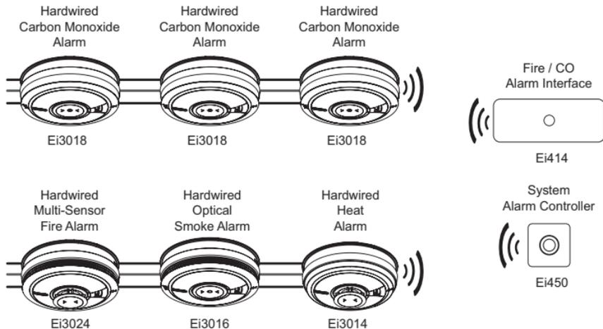
The hardwired interconnected sections of a hybrid system should be separated into CO only Alarms and Fire, Smoke and Heat Alarms, to ensure that the alarm type is indicated correctly to the RF network during activation
