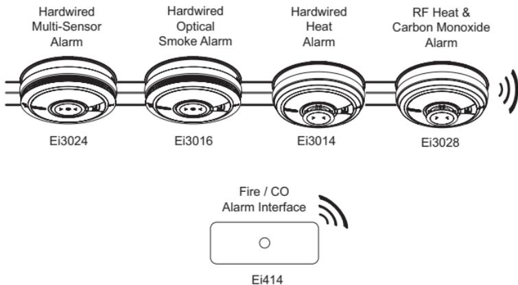
If an Ei3028 Heat and CO Alarm is required on a hardwired section, it should be fitted to a Fire, Smoke and Heat only section, one per section and that Ei3028 should also be the section's link to the RF network of the hybrid system. This ensures that the RF Fire alarm message can be transmitted if any device on the hardwire circuit is activated and the RF CO Alarm message if the Ei3028 detects dangerous levels of CO
