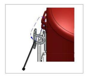
5. Attach the extinguishing agent container to the intended retaining bracket with a cable tie
