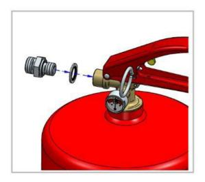
1. Screw hose adapter including sealing ring into extinguishing agent container and tighten (30 Nm)
