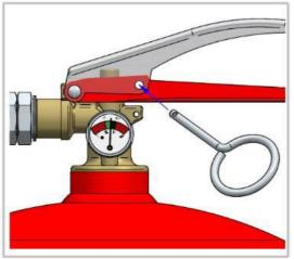
8. Insert the locking pin in the pressurized position of the lever armature
