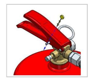
9. Lock the locking pin using the plug-in seal
