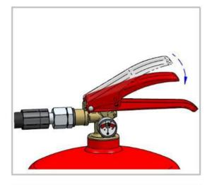
7. Actuate lever armature ---> Extinguishing system is now under pressure!
