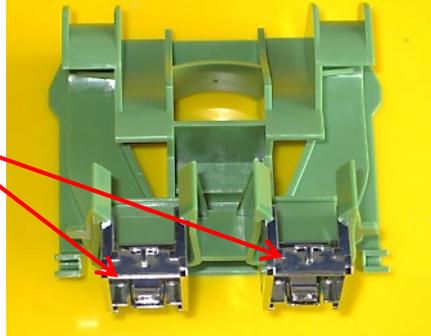
2. Make sure that the 2 hocks of the Keystone adapter fit into the 2 cavities of the green module fixing.
