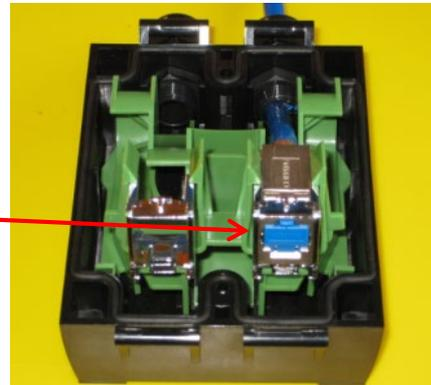
4. Remove the dust cap from the xs500 module.
