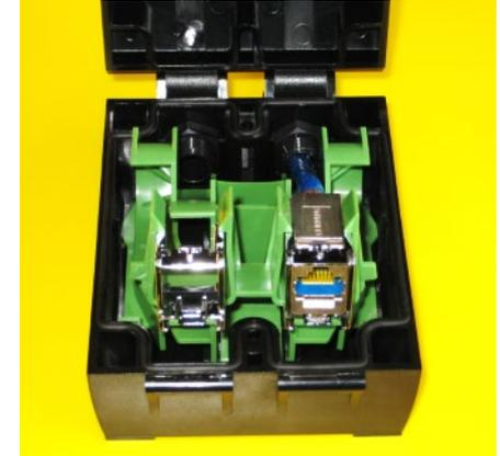
5. Install the cover and the dummy plug into the non used cable entry.
